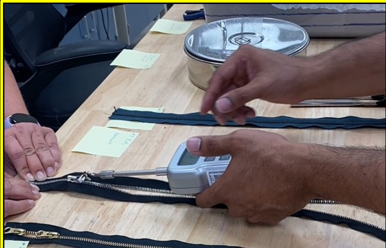
Measuring actuation forces of zippers pre and post-application of lunar simulant.
