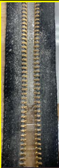
Measuring actuation forces of zippers pre and post-application of lunar simulant.
