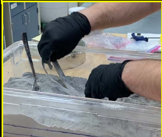
“Dunk Test” Zipper is fully immersed in simulant
