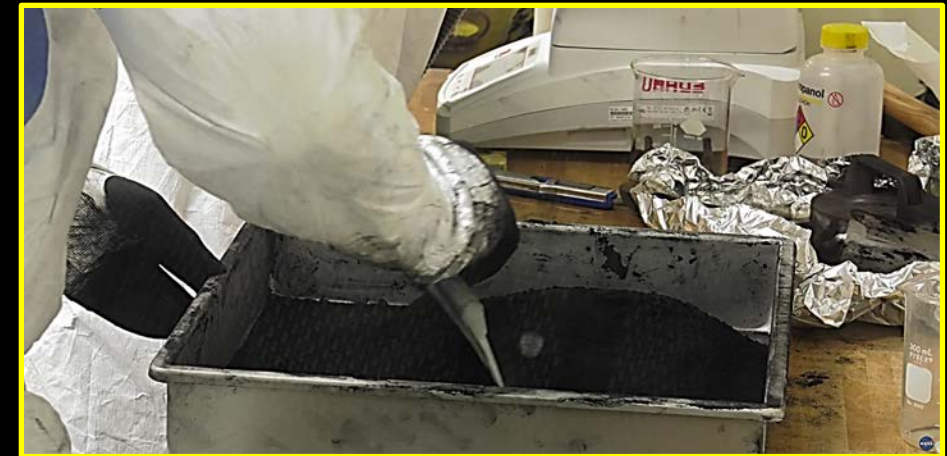
preparing the regolith simulant for oxygen extraction
